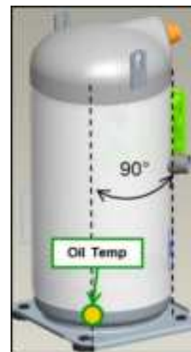
Figure 17: Oil dilution chart ( t_b = bottom shell temperature; t_e = evaporating temperature) and position of oil temperature sensor
