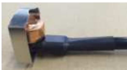
Figure 10: Discharge line thermostat with clamp
