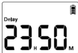
Rain delay allows you to postpone watering for a set period of time, and it doesn't interrupt your original schedule.
