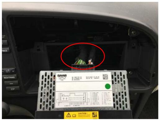
Step 4) Separate the ICM connector by lifting the plastic lock and slide out the sub-connector (be careful not to damage the fiber optic cable)
