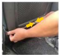
STEP2: Pull the side straps to the backside.
