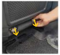
STEP1: Push the <u>chuck</u> (③) into the gap between bottom seat and backrest, and get <u>them</u> (③) from the backside.
