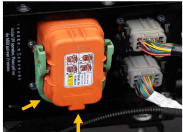
Image: MSD slide switch & green handle
