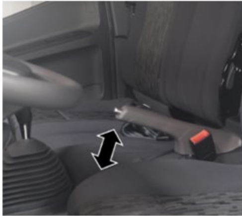
Image: Parking Brake Engaged
