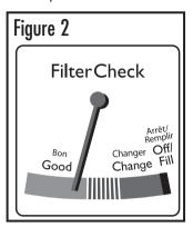
When the needle is in the red (CHANGE) section, this means the proper amount of moisture is not getting into your air due to the excessive minerals and sediment that have become trapped on your filter. At this point, you should replace your filter. It is important to change your filter as indicated to obtain stated performance level.
