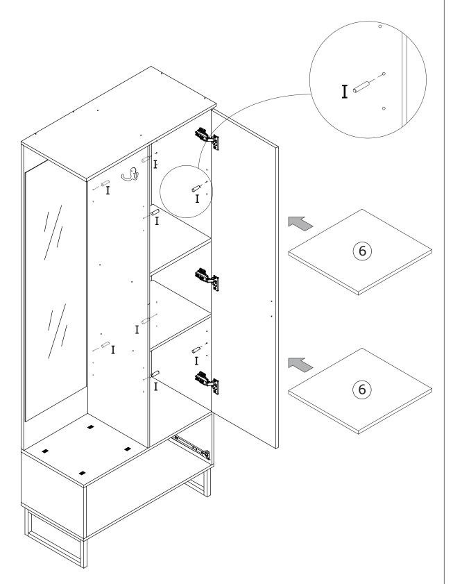
Insert the shelf pin(I) to the panel as shown, then put the panel #6 on the shelf pin.
