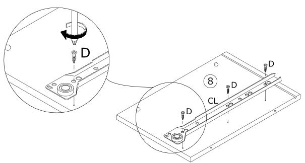
Using 3pcs screws(D) to lock the slide(CL)
