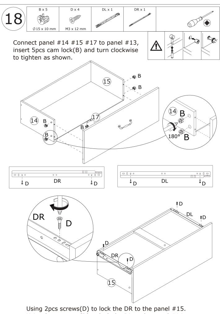
Using 2pcs screws(D) to lock the DL to the panel #14.
