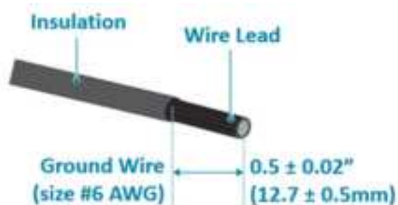
6-AWG green-and-yellow wire for grounding
