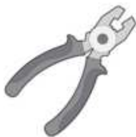
Wire-stripping tools for stripping 6-AWG copper wire
