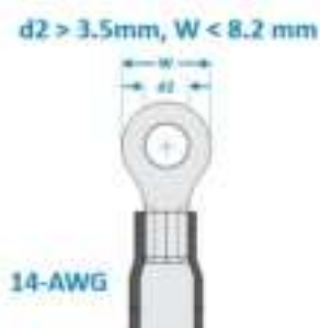
14-AWG wire with ring terminal for DC power supply
