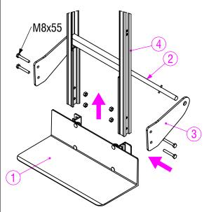
Please follow →direction for assemble. 1 nose plate 2 axle 3 axle boxes the axle should go throuth the axle boxes then, the axle boxes throuth be combird with hand truck body
