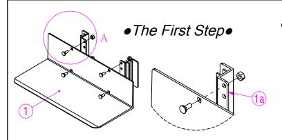
The screw according to the line direction to go through the hole and lock with 1 toe plate and connection.
