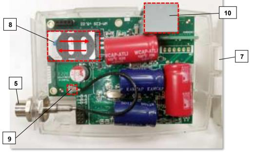
Step #6: Insert a replaceable and active SIM card (with APN access) into the SIM-holder (8) -
