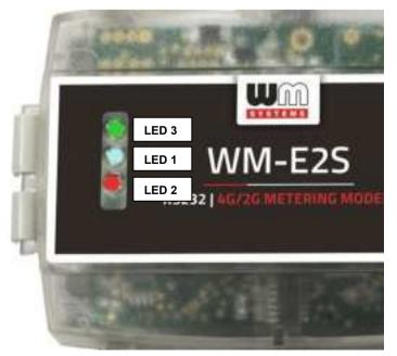
At the first power on - during the charge - the green LED is flashing quickly. After a few minutes the LED will be blank, then qill be flashing quickly again. When the green LED will be flashing slowly and the other LEDs will be lighting according the NORMAL operation, then the modem will be charged completely and it will be ready for congfiuring and to operate.
