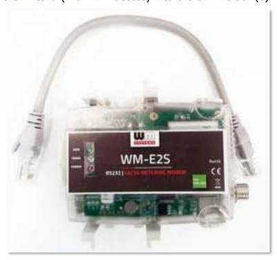
Step #9: Close the top of the enclosure – taking care of its exact positioning on the lugs and holders - until it is fastened (you will hear a click when it is closed).
