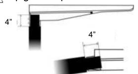
Open luminaire only if base is supported or if luminaire is installed on the pole
