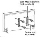
If using an electric screwdriver, set the torque at approximately 1.5 N·m {15 kgf·cm}.
