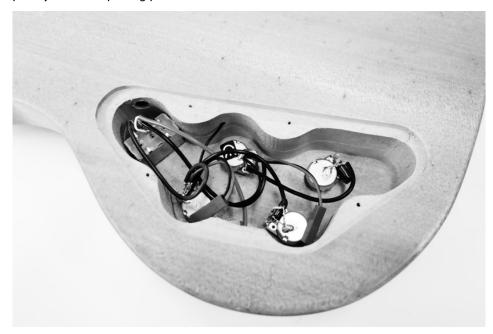
Screw the potentiometers finger-tight to the body surface with a washer and a hex nut each.
