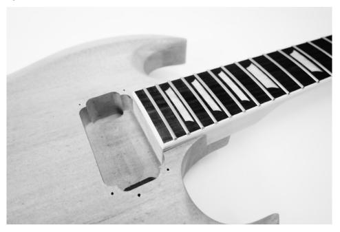
Turn the guitar over, position the mounting plate over the four screw holes on the back of the body and screw the four supplied long wood screws through the holes in the mounting plate into the body and neck until the connection is firm.
