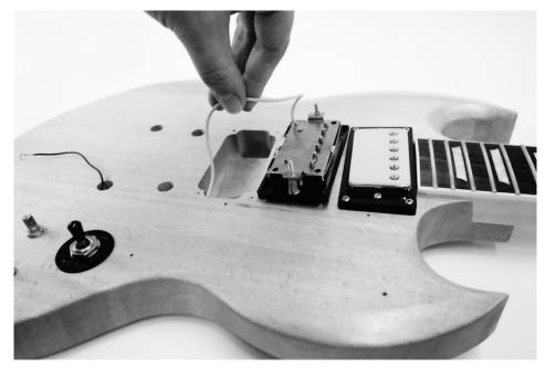
Connect the plugs to the potentiometers: The upper tone and volume potentiometers are generally connected to the neck pickup, and the lower tone and volume potentiometers to the bridge pickup.
