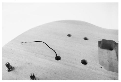
Then insert the potentiometers into the opening in the back as shown and wire the potentiometers to the switch. Guide the switch from the back of the body completely into the opening provided for it.
