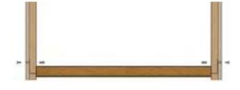
3. Secure the Angle Brackets with Joint Connectors: Repeat the process to tighten the joint connectors. Once aligned, fully tighten all connectors, ensuring the connectors do not interfere with the NC boards (do not over-tighten).
