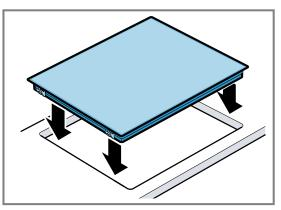
The hob can also be installed in an existing cut-out that has a depth of 500 mm.
