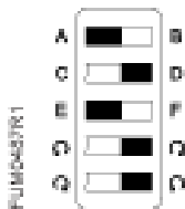
Switch Settings for the Fast Acting Lab Electronic Actuator.
