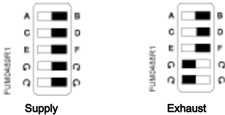
Switch Settings for the Fast Acting Lab Electronic Actuator.
