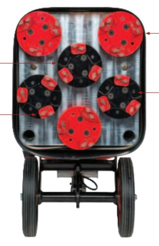
COUNTER-CLOCKWISE SPINNING RHINO TOOL PLATES (RED)
