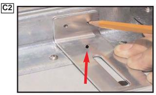
Install additional #6 screw here if desired
