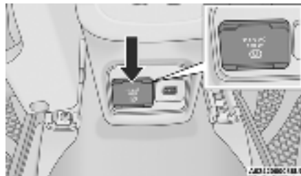
Power Inverter Location
