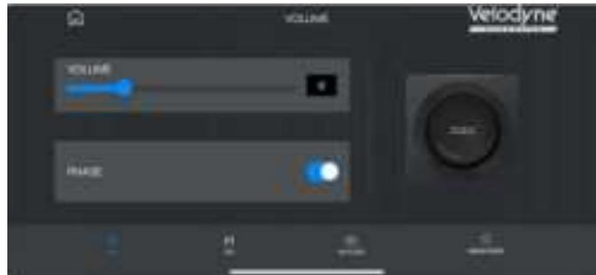
2. Volume Control – adjust the subwoofer level by sliding the control dot from 0 to 30
