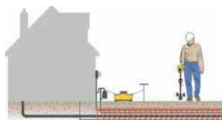
Direct connect to utility lines
