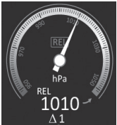
Pressure rising or falling rate in 3 hours
