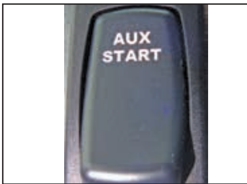
Figure 8-2: Auxiliary start switch
