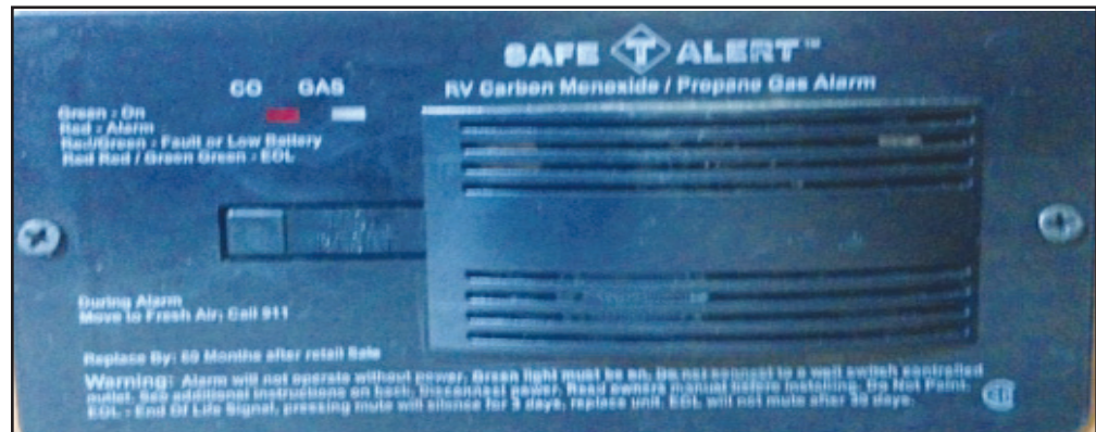
Figure 2-3: Carbon Monoxide alarm
