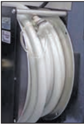
Figure 12-4: City water supply connection
