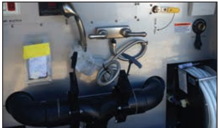
Figure 12-8 Sanitation coupling, valve and hose
