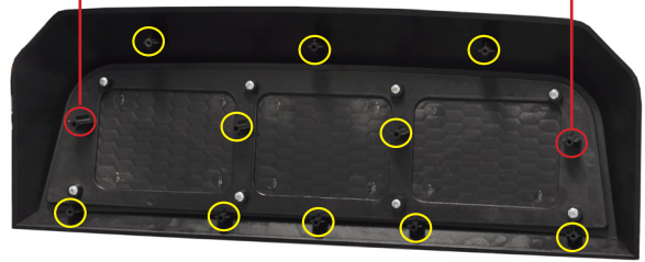
Here are the mounting locations on the back side of grill
