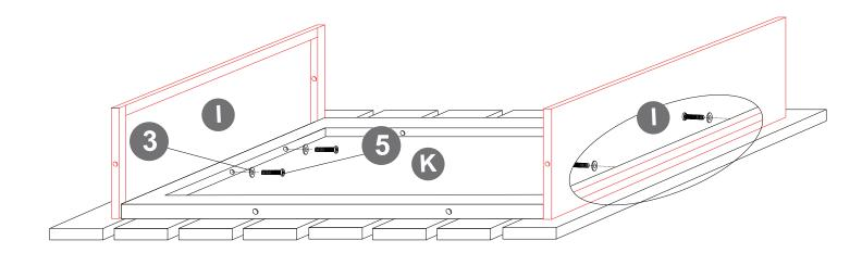
Tighten the screws 40% to proceed to the next step in the installation.
