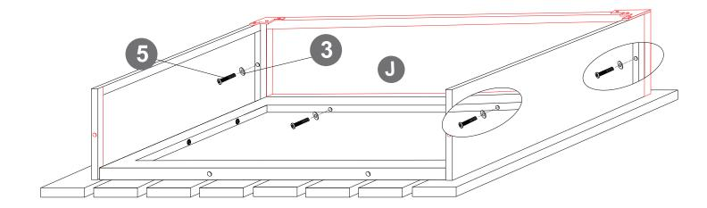
Tighten screws 40% and all screws when finished.
