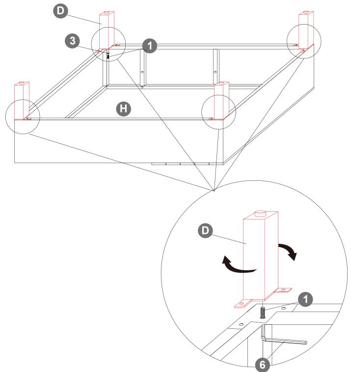
After tightening the screws, tighten the bottom screws
