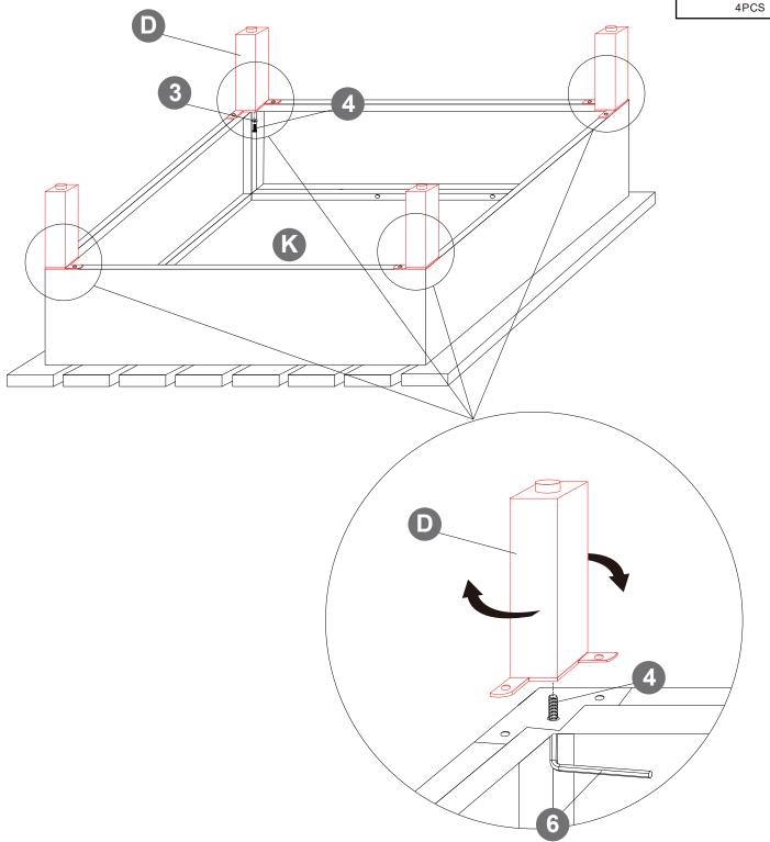
After tightening the screws, tighten the bottom screws.
