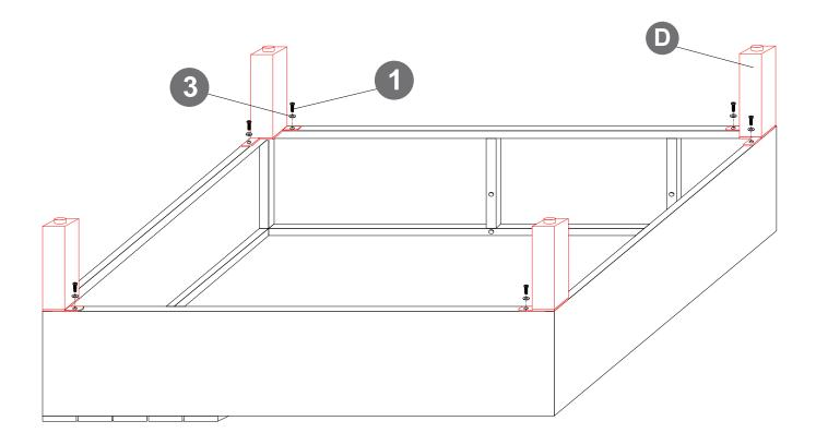
Align holes by placing part C under part G to make installation easier. Tighten the screws 40% to proceed to the next step in the installation.
