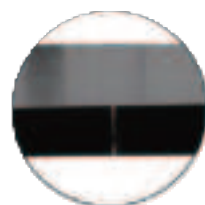
Hemming process results, Not broken here
