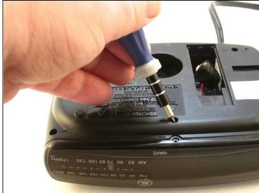
• Using a Phillips #00 Screwdriver, unscrew the six 12mm screws from around the bottom of the clock radio.
