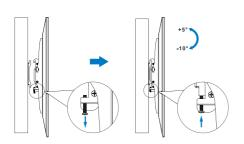
Apply the TV with wall mount to the wall plate
