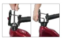
Install the top cap and bolt onto the head tube. Ensure there is no gap between the stem and head tube by pressing them together while tightening the top bolt. This prevents wobbling during use. If wobbling occurs, repeat this step.
