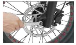
3 Securely tighten the axle end nuts.
