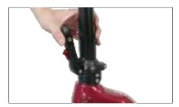
4 Apply downward pressure on folding lever until lock engagement is confirmed.
