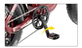
2 Gently thread the right pedal onto the right crankarm clockwise. Then, use an open-end wrench to tighten the pedal.
