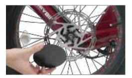
Extract the axle protector caps from both ends of the front wheel hub.
