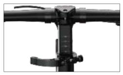
To adjust the handlebar, pull open the clamp on top of the stem. Set the handlebar to your desired height, then close the clamp securely. If the clamp feels too loose or too tight, adjust the clamp side bolt as needed.
