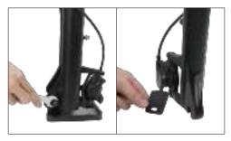
1 Detach the fork protector, extract the brake pad spacer clip from the caliper assembly.
