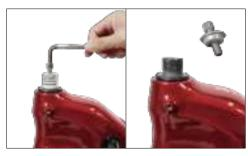
1 Loosen and remove the top screw and protective ring mold. Keep the top bolt and cap for reinstallation.
