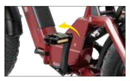
Gently thread the left pedal onto the left crankarm counter-clockwise. Then, use an open-end wrench to tighten the pedal.
