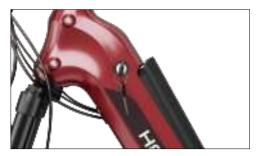
Ensure the bike is turned off. Insert the battery key and turn it counterclockwise to unlock the battery. The battery will pop out once unlocked.
