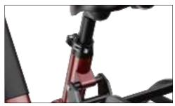
Close the quick release lever using your palm or finger. If the clamp feels too loose or tight, adjust using the clamp side bolt.
