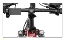
Ensure the handlebar is facing forward and aligned perpendicular to the front fork.
