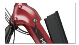
2 Hook the battery with your hand and lift it upward to remove.
