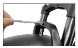
1 Remove the headlight bolt from the front fork, insert the fender under the fork with the longer end covering the rear side of the wheel.
