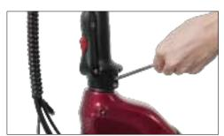
Tighten the two lower side bolts on the stem.
