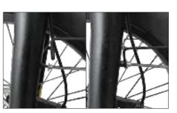
3 Remove the screws located on the sides of the front fork, near the spokes, align the fender stays with the openings, and secure them by tightening the bolts.
