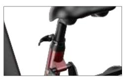
Move the seat up and down by sliding the seatpost in or out of the seat tube. DO NOT raise the seatpost beyond the minimum insertion marking etched into the seatpost tube.
