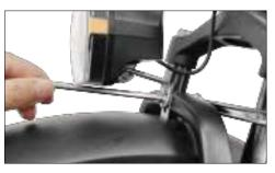
Align the holes of the fender, headlight bracket, and fork, then reinstall and tighten the headlight bolt with a washer on each end between the nut and the fork.
