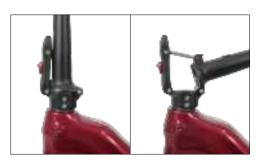
Slide the stem onto the steerer tube. While maintaining upward thumb pressure on the folding lever's release mechanism, pivot the lever outward to extend the stem.
