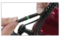
4 Connect the headlight plug by aligning the arrows and pushing straight in without twisting. You may need to open the wire sleeve to locate the connector.
