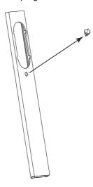
4 Install a 1/2 in. inside diameter drain hose on the back of the unit where you removed the rubber plug. Use a hose clamp to make sure that there are no leaks.
