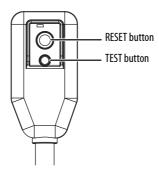
The circuit breaker should be tested periodically by pressing the **TEST** button then the **RESET** button. If the **TEST** button does not cause the circuit breaker to trip, or if the **RESET** button does not stay engaged, unplug the air conditioner immediately and contact an Insignia technician.
