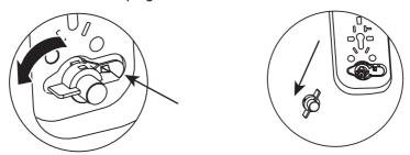
**3** Remove the rubber plug from the window plate.
