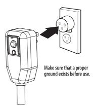
To prevent damage to the adapter's ground terminal, hold the adapter in place while plugging or unplugging the air conditioner.
