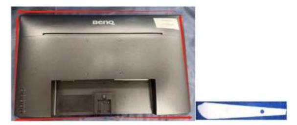
c) Disconnect cable to remove back cover.
