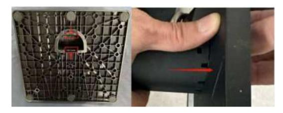
b) Use the sharp object to press the protruded object, and hold the stand with the other hand to push it downward until the stand detached.
