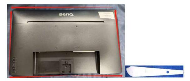
c) Disconnect cable to remove back cover.
