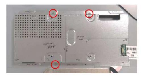
c) Lift up main frame and disconnect cable to remove it.
