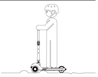
Keep your speed between 3-6 mph when you ride through speed bumps, elevator door sills, bumpy roads or other uneven surfaces. Slightly bend your knee to better adjust mentioned surfaces.
