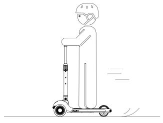
3. The motor will engage when the scooter is travelling to 1.9 mph (3 km/h).
