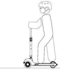
5. For controlled stops, apply the brake by putting pressure on the rear fender brake.
