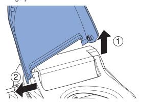
Remove the left hinge pin and pull the WC seat ring slightly forward.
