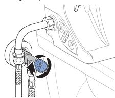
2 Loosen the connection bend and empty the residual water into a receptacle.
