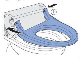
9 Push in the left hinge pin and let it snap into place by turning it.
