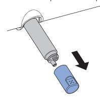
4 Replace the spray nozzle if it can no longer be completely cleaned and descaled.
