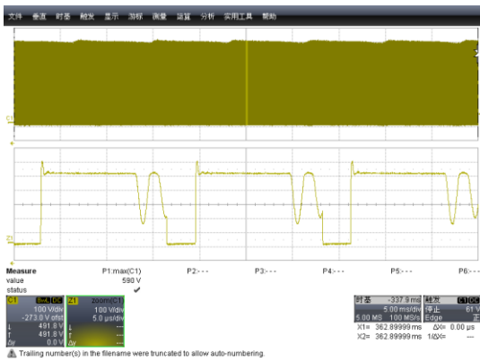
Figure 14: Q1 Vds=590V Vdsmax=650V, Trv = 90.8%
