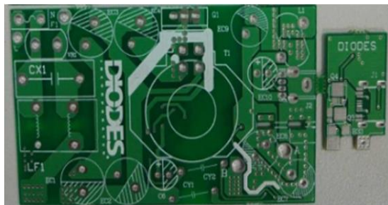
Figure 6: PCB Board Layout Top View
