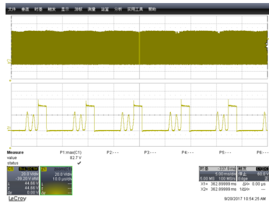
Figure 15:Q2 Vds =82.7V Vdsmax=100V Trv = 82.7%
