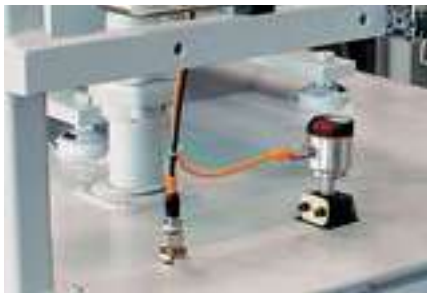
ifm's electronic LK level sensors can be inserted into a tank opening as small as 20 mm in diameter.
