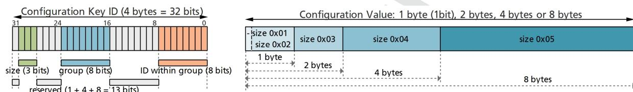
A Configuration Key ID is a 32 bits integer value, which is split into three parts (Note that bits 31, 27..24 and 15..8 are reserved for future use and are currently unused.):
