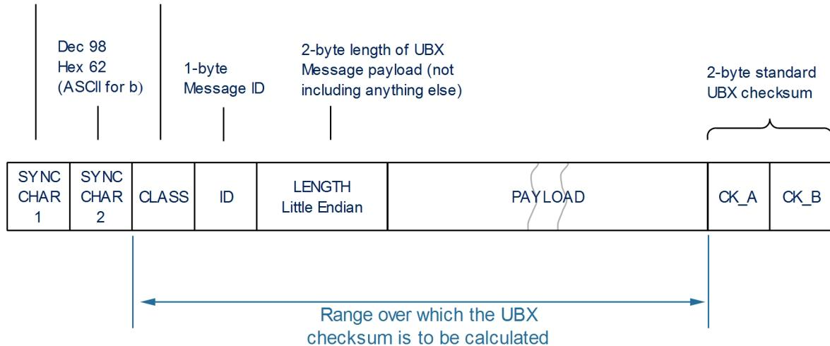
The checksum algorithm used is the 8-Bit Fletcher Algorithm, which is used in the TCP standard ([RFC 1145](#)). This algorithm works as follows:
