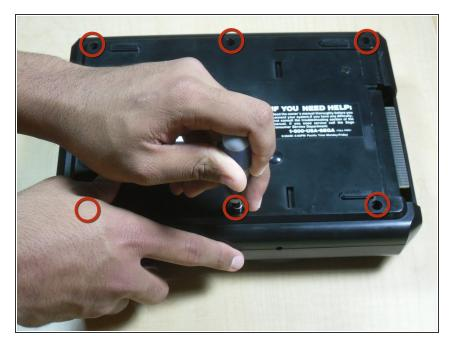
Remove the six screws from the underside of the console with a Phillips #1 screwdriver.
