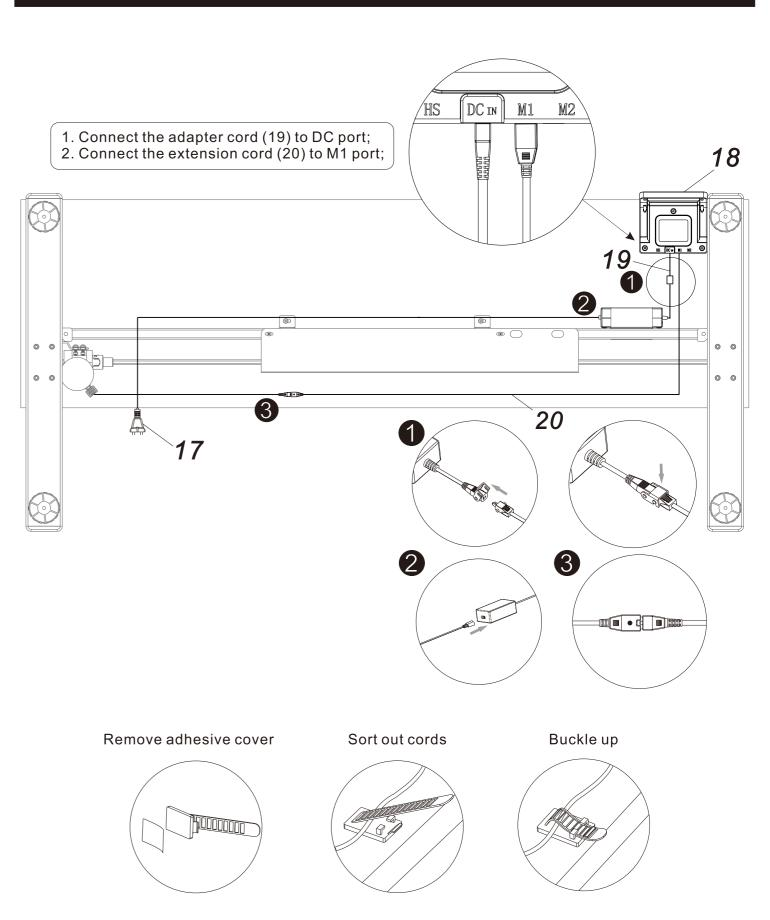
The cable tie (I) can be used to fasten the cables to the desktop.
