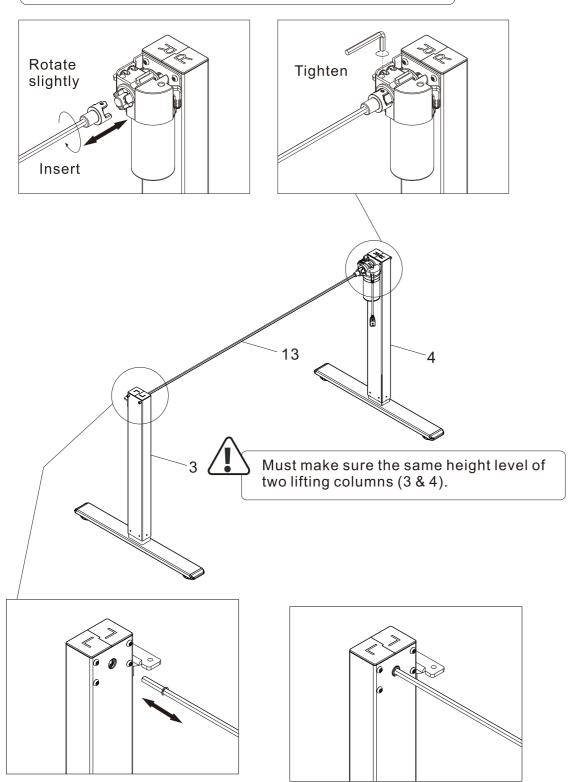
Note: Please insert the transmission rod until shaft stopper touches the column.
