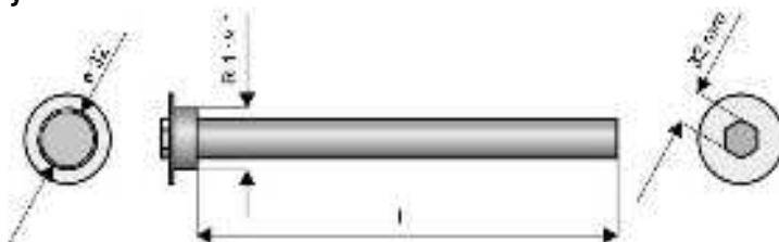
Insulated magnesium anode - connection size and length
