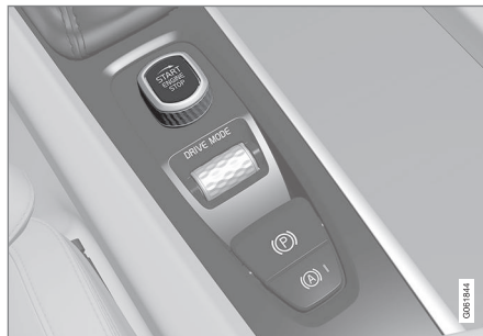
Start knob in the tunnel console.
