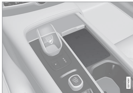
Wireless phone charger in the tunnel console.
