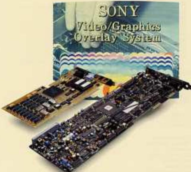
The SONY VGA Video/Graphics Overlay System is a high-resolution, non-interfaced graphics system and video-overlay board set which meets and exceeds industry graphics standards by offering a variety of graphic and character display modes including CGA/EGA/VGA and Advanced VGA. The two-slot computer card set can be added to any IBM® PC™, PC-XT™, and PC-AT™ compatible computers.
