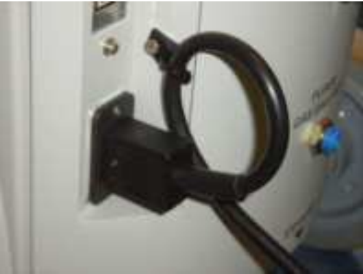
Fig. 6: Mains cable with fixing
