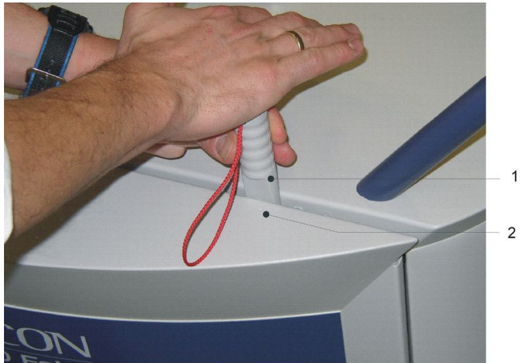
Fig. 30: Opening the UL1000 / UL1000 Fab
