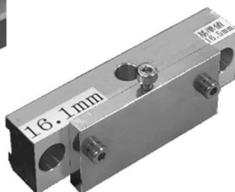
Track position check jig (Refer to p.24 for Dimensional diagrams)
