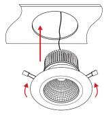
Bend springs upward and install luminaire into ceiling. Once installed the springs should clamp down on the ceiling to support the fixture.
