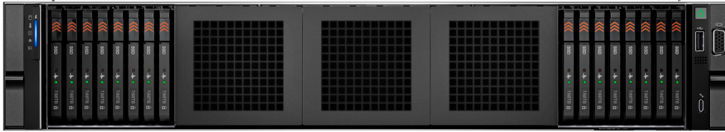
Figure 5. Front view of 16 x EDSFF E3.S Gen5 NVMe drive system
