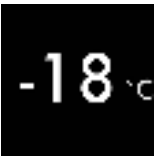
Fig. 6 (1) Temperature display The Status displays the set temperature. From there, you can navigate to the functions and settings.
