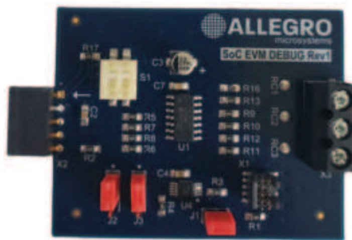
Figure 3: A892xx Universal Debugger
