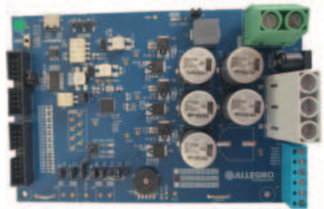
Figure 1: A89211/2 Evaluation Board
