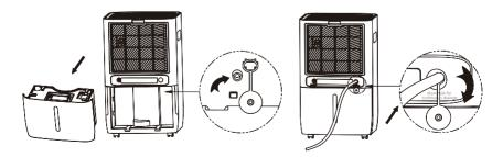
⚠ **WARNING:** the end of the hose should not be submerged in water to prevent it from being blocked or damaged.
