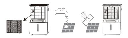
**WARNING:** It is strongly advised to rinse the filter every two weeks. Any dust blocking the filter will potentially affect the machine's functionality.
