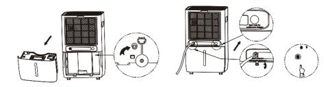
MARNING: the end of the hose should not be submerged in water to prevent itfrom being blocked or damaged.
